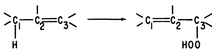
Figure 1. Primary products from olefin photo-oxygenations, showing unsaturation in position adjacent to original position
